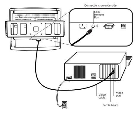
• Connect the 6 pin DIN cable to the OSD Remote port on your touchmonitor.
